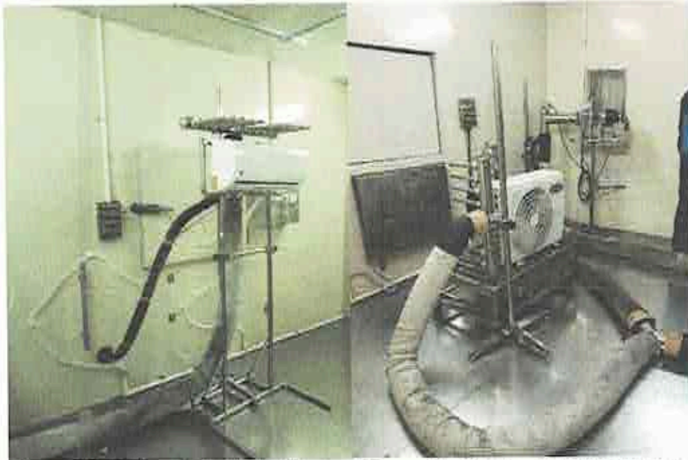
Figure 2a. Indoor Unit Under Test Figure 2b. Outdoor Unit Under Test
